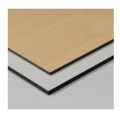
EGGER compact laminates black core are compact laminates according to EN 438-4, respectively EN 438-8 with a black core, based on curable resins. They have a multilayer structure and consist of melamine resin impregnated decorative paper and multiple layers of soda kraft paper impregnated with phenolic resins, which are laminated under high pressure and heat.
